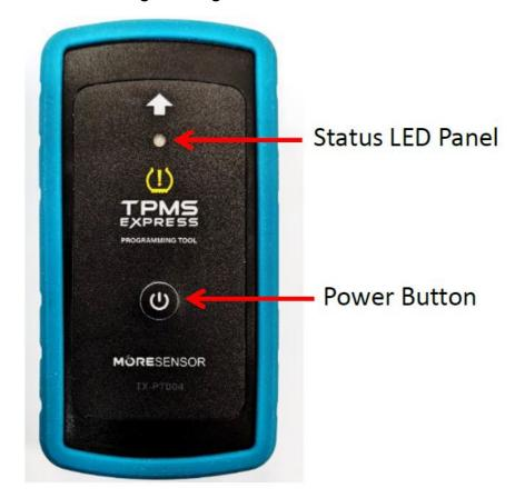
The TX-PT004 is controlled using an application installed either on an iOS or Android device through the "TPMS EXPRESS" application. Bluetooth capability is required for smartphones and tablets.
