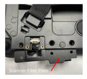
4. Install the Scanner Filler Plate.
