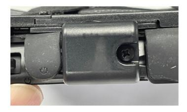
10. Install the M3 x 5 Pan Head screw.
