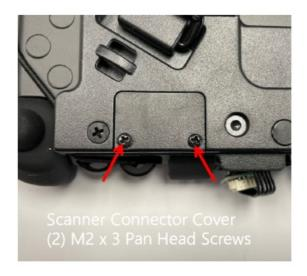
6. Install the Scanner Connector Cover using (2) M2 x 3 Pan Head screws.
