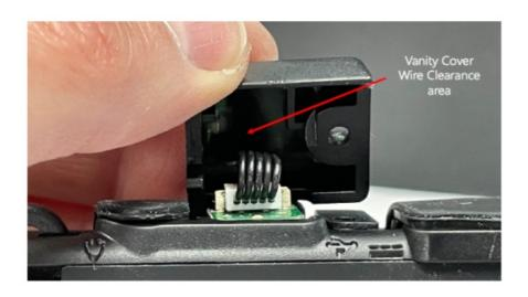
9. Install Vanity Cover over USB Type C PCB. Ensure wires are aligned in Vanity Cover clearance area so that wires are not pinched.
