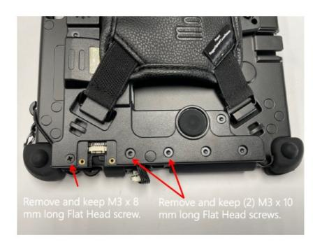
3. Remove M3 x 8 & (2) M3 x 10 Flat Head screws.
