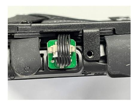
8. Plug USB Type C PCB into USB Type C connector as shown.
