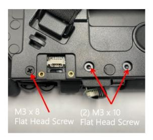
5. Re-install the M3  $\times$  8 and (2) M3  $\times$  10 Flat Head screws.
