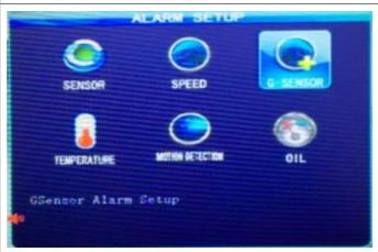
4) On the G-Sensor Setup page, use arrow keys to hi ghlight Enter button to the right of the X, Y, and Z sen sor values. Press Return and watch that the values ar e now approximately 0.
