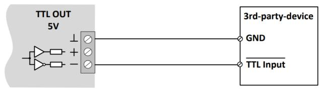
Signal inversion by using the negative signal output
