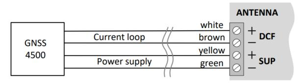
The current loop-voltage corresponds to the DC input voltage (DC IN), but it is limited to 30V, if input voltage is higher.
