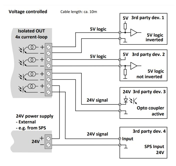
Wiring of the TTL Output
