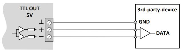
Both signal outputs used (pos/neg) and reference GND cable length: <1km
