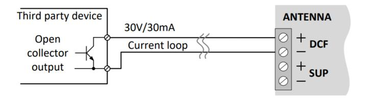
Wiring of the optocoupler outputs
