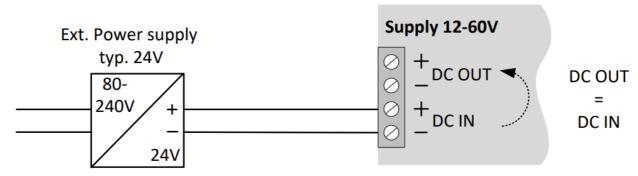
DC-supply 12V to 60V over external power supply or from a third party device.
