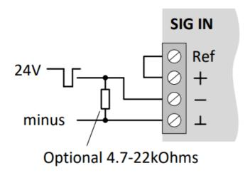
Wiring receiver input (current controlled)
