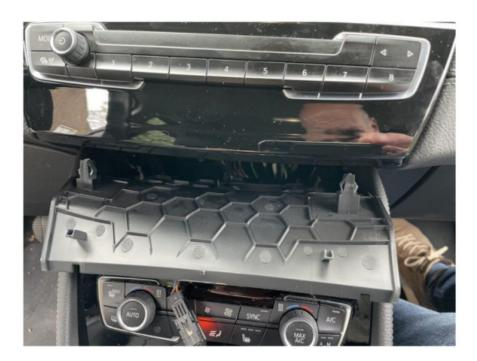
**Step 2.** Remove the control panel from the radio (screw and unclip)
