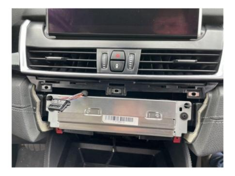
**Step 3**. Remove the front panel with the air vents (unclip)
