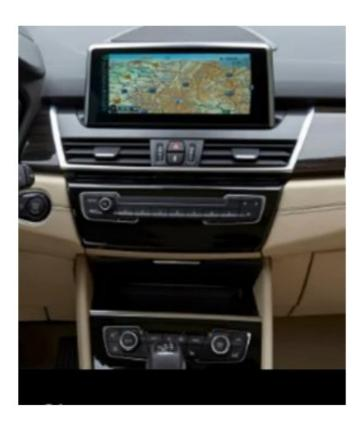
**Step 1**. Remove the front panel underneath the radio (unclip)
