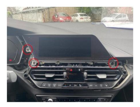
Step 3. Remove the panel with the air vents (screws)
