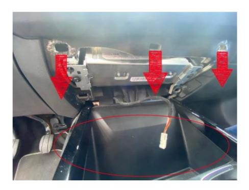
Step 5. Remove the head unit (screws)
