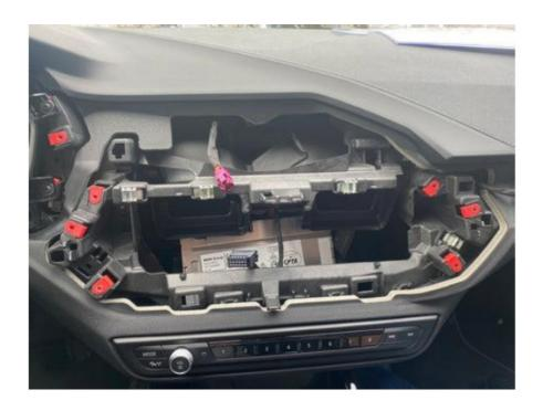
Step 4. Remove the panel under the control unit from the radio (unclip) Unclip the panel.
