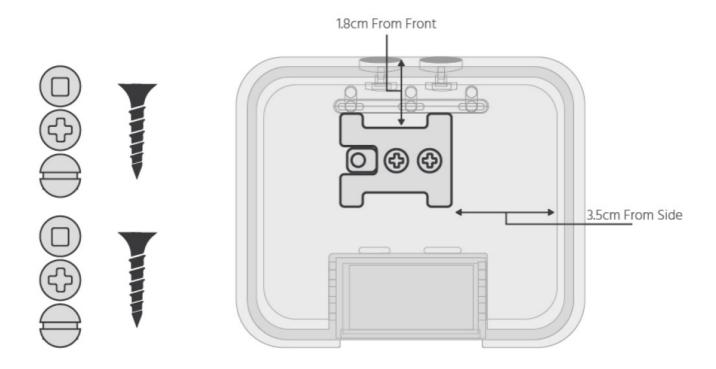
**Caution:** Do not overtighten screws. Screws must be flush with the mounting bracket. # 4 Flat Head screws only. The mounting bracket should be level and installed flush to the wall or ceiling surface material.
