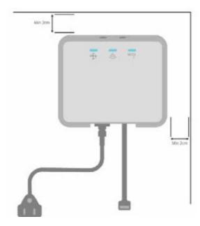
The MMB TME can be mounted on walls or ceilings. The ideal orientation is vertically on a flat wall, with Power and Ethernet cables facing down. A clearance of 2cm on all sides should be maintained.
