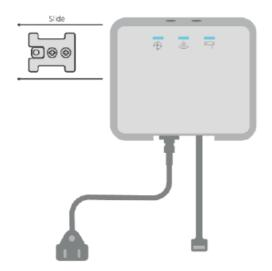
Once the mounting bracket is correctly installed, and with Ethernet and Power cables connected to the MMB TME, slide the MMB TME onto the bracket from left to right to mount.
