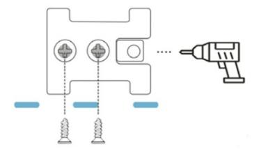
**Caution:** Do not overtighten screws. Screws must be flush with the mounting bracket. Use # 4 Flat Head screws only. The mounting bracket should be level and installed flush to the wall or ceiling surface material.
