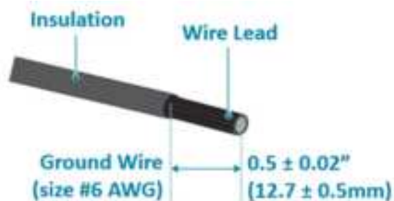
6-AWG green-and-yellow wire for grounding
