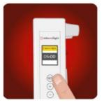
• From the Home Screen press 'SET' to navigate to the Settings Screen. To adjust the Default Time, Mode, Bluetooth connectivity, and Brightness settings press 'SET'.
