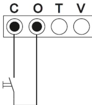
Push-button to be used: normally open contact
