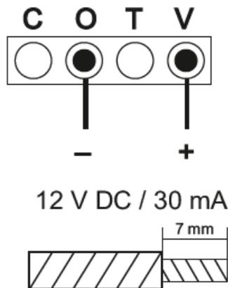
Strip the individual wires 7 mm and connect them to terminals (V) = + and (O) = -
