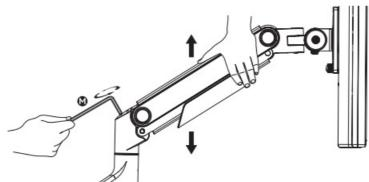
To properly balance the arm with the monitor stand, adjust the spring tension using the supplied Alen key as follows:
