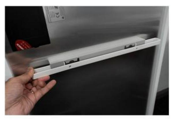
• Step 7: Ensure that both lips of the ceiling bracket fit into the frame holes on both sides, like shown in the picture below
