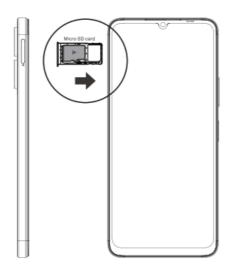
**Caution:** Please use standard nano-SIM card only. Non-standard SIM or hand-cut SIM card may damage the SIM tray or phone and causes SIM rejection situation. Always turn off the phone before installing or replacing SIM cards or a micro-SD card.
