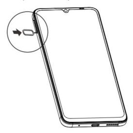
• Put 1 or 2 nano-SIM cards onto the SIM tray with the gold contacts facing down and the notched edges match the positions on the SIM tray.
