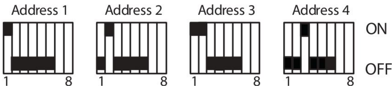
Figure 3 Set the RS-485 address
