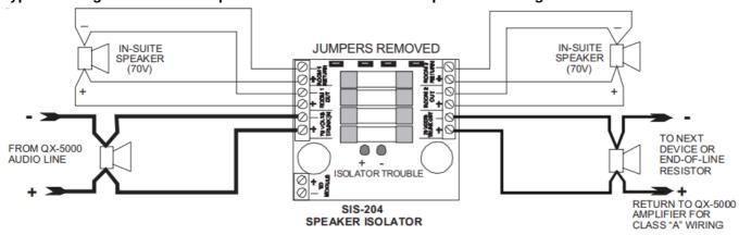
THE (+) LED WILL BLINK FOR AN OPEN ON THE POSITIVE SIDE OF THE IN-SUITE SPEAKER, SIMILARLY, THE (-) LED BLINKS FOR AN OPEN CIRCUIT ON THE NEGATIVE SIDE OF THE IN-SUITE SPEAKER.
