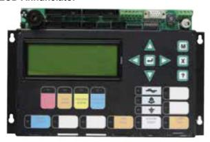
The RAXN-LCD Remote Network LCD Annunciator is equipped with a large 4 line x 20 character back-lit alphanumeric LCD display that provides an exact replica of the main FleX-Net fire alarm control panel display. The RAXN-LCD occupies one display position in the BBX-FXMNS, BB-1000 or BB-5000 series enclosures.
