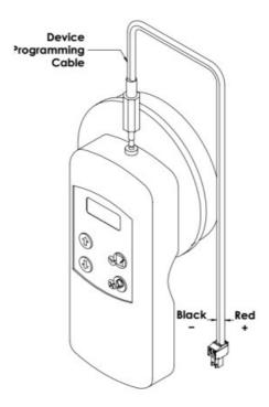
Unless the device has to be replaced, there is no need to disconnect wires from it. However the whole SLC line should be disconnected from the loop driver when devices are programmed while in place. If the SLC line is powered, the programmer may be unable to read or write the device data.
