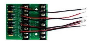
**OCAC-304 Four Indicating Circuit Class "A" Converter Module** The OCAC-304 converts four Class "B" (Style "Y") indicating circuits on the FA-300 main board to Class "A" (Style "Z") circuits. The OCAC-304 is equipped with wire leads to connect to the FA-300 main board. It mounts to the right of the main board Class "B" (Style "Y") indicating circuits and is used with the FA-301-12DDR series panels.
