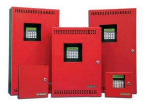
Mircom's FA-300 Series fire alarm control panels consist of 6 and 12 zone models which are equipped with a two line by 20 character back-lit LCD display, numerical keypad and an integrated UDACT/Digital Communicator. The FA-300 Series family also includes remote LED and LCD annunciators as well as remote relay modules.
