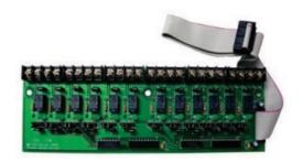
ICAC-306 Six Initiating Circuit Class "A" Converter Module The ICAC-306 converts six Class "B" (Style "B" initiating circuits on the FA-300 main board to Class "A" (Style "D") circuits. The ICAC-306 is equipped with wire leads to connect to the FA-300 main board. It mounts to the right of the main board Class "B" (Style "B") initiating circuits. Two ICAC-306 modules are required to convert all twelve initiating circuits on an FA-301-12DDR series panel.
