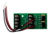
**OCAC-302 Two Indicating Circuit Class "A" Converter Module** The OCAC-302 converts two Class "B" (Style "Y") indicating circuits on the FA-300 main board to Class "A" (Style "Z") circuits. The OCAC-302 is equipped with wire leads to connect to the FA-300 main board. It mounts to the right of the main board Class "B" (Style "Y") indicating circuits and is used with the FA-300-6DDR series panels.
