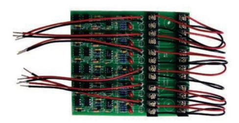
ICAC-306 Six Initiating Circuit Class "A" Converter Module The ICAC-306 converts the six Class "B" (Style "B" initiating circuits on the FA-300-6DDR-CG main board to Class "A" (Style "D") circuits. The ICAC-306 is equipped with wire leads to connect to the main board.
