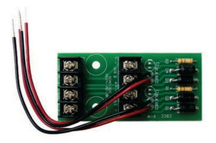
OCAC-302 Two Indicating Circuit Class "A" Converter Module The OCAC-302 converts the two Class "B" (Style "Y") notification appliance circuits on the FA-300-6DDR-CG main board to Class "A" (Style "Z") circuits. The OCAC-302 is equipped with wire leads to connect to the main board.
