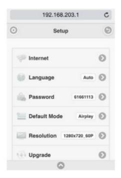
After WiFi is connected with MiraScreen, you can open your web browser to edit settings, please enter IP: 192.168.203.1 (Sample fig. is based on mobile device)
