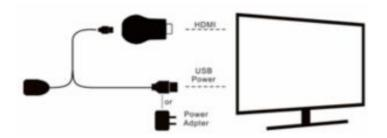
Due to 802.11 b/g/n WiFi module will consume more power, please be noted to use a power adapter with at least 1Amp supply (5V1A adapter is recommended)
