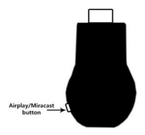
AirPlay/Miracast button: Switch AirPlay or Miracast Mode on the fly
