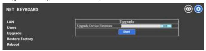
Choose the right upgrading file and click "start" to update the controller. It will auto reboot after updating. **PS:** Do not operate the controller during the upgrade process. Do not power off or disconnect network
