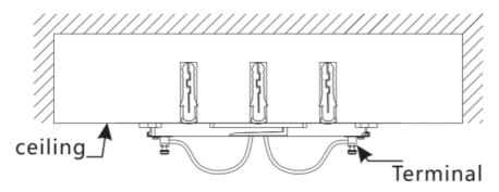
5. The arrow on the back of the lamp is aligned with the one on the fixing bracket arrow, turn clockwise for 45 ° to clamp
