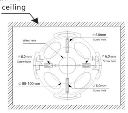
3. After drilling the expansion screws into the screw holes, using the screws to fix the fixed frame
