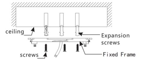
4. Take out the wires from wire hole, connect the L wire and N wire as shown on the fixed frame with the stud screw, screw tightly. This lamp is made of plastic, Earth wire is unnecessary)
