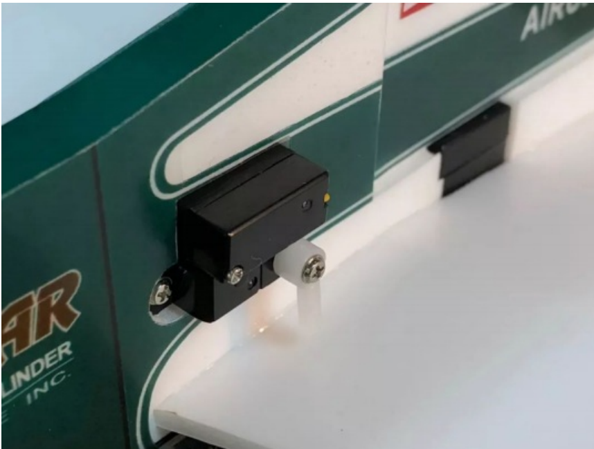
19. Connect the pushrod clips & pushrods with heat shrinkable tube and fix them with glue.
