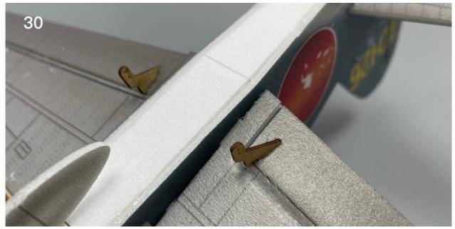
Install rudder control horns.
