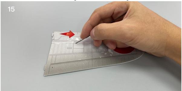
Use the end of a carbon fiber rod to score through the aileron half-cut line of the wing surface.
