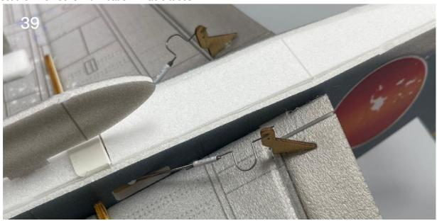
Paste the carbon fiber rod at the broken line at the bottom of the wing to increase the strength.
