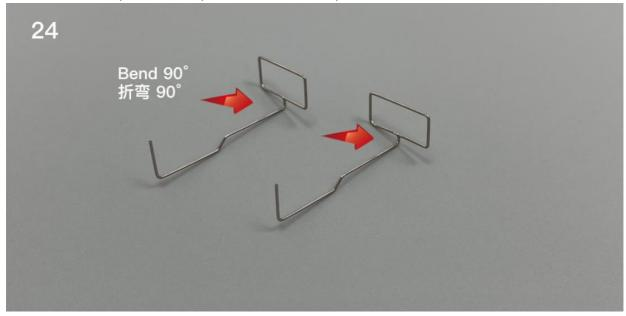
bend the outer end of the steel wire with pointed nose pliers.
