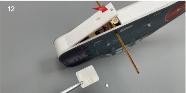
The battery cover can be opened, and can be adsorbed in the closed position by magnet.
