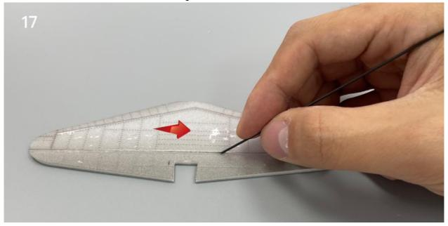
Use the end of a carbon fiber rod to score through the half-cut line of the rudder surface.
