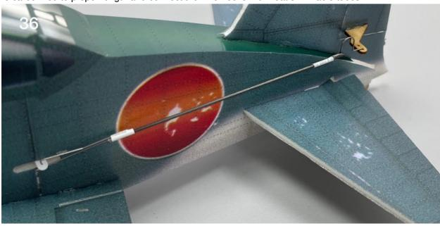
Use heat shrinkable tube to connect aileron steel wire clips.
