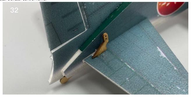
Use heat shrinkable tube to connect tail push rod and steel wire clip.
