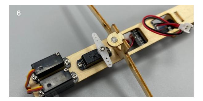
Align the scribed line on the inner side of the fuselage and fix the wooden structure with glue.
