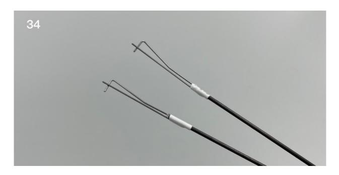
Attach the steel wire hooks to the control horns.
