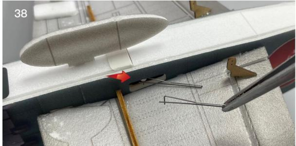
Connect the wire hooks with heat shrinkable tubes.
