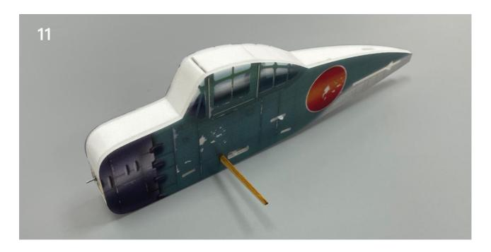
Fix the battery cover magnet with glue and cover it with stickers.
