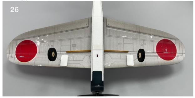
Fix the landing gear cover plate with circular stickers, which can be reinforced with glue.
