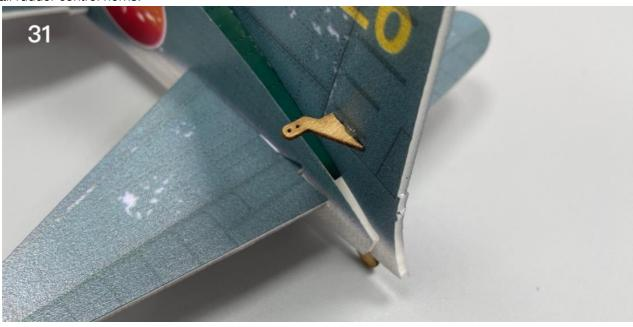
Install elevator control horns.
