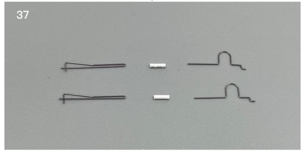
Attach the steel wire clip to the aileron servo arm.
