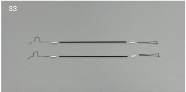
Use heat shrinkable tube to connect the pull rod and wire clip, then use glue to fix them.
