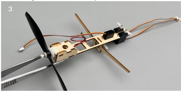
(bottom view) the three servos are installed and fixed under the plywood board.
