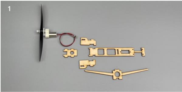
Bond the inner structure of the fuselage with 502 glue.
