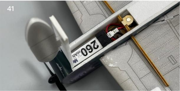
Optional accessories: pilot. Cut off the cockpit cover along the scribed line and install the pilot base and pilot. **Note:** the installation pilot will change the vertical center of gravity of the aircraft. It is recommended to remove the pilot during flight.
