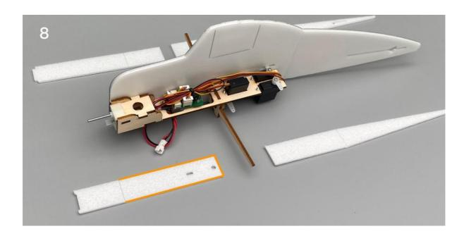
Cut out the illustrated orange area on the sticker to avoid interference with the motor gears.
