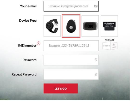
2. Before starting the tracking for the first time, please make sure to place the device outdoors for 3-5 minutes for faster fixing against GPS satellites. Start the device by plugging it into the charger.
