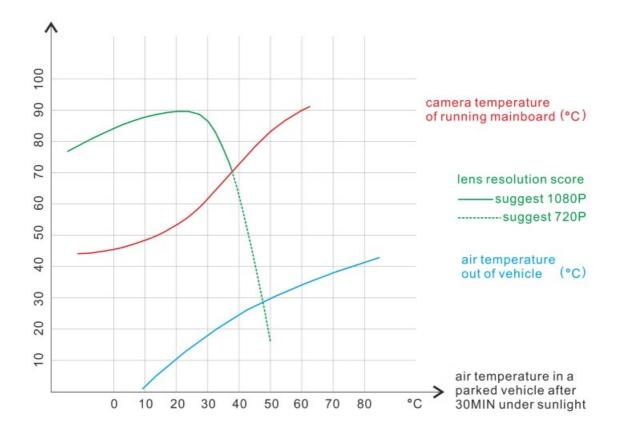
Air temperature & in vehicle temperature & camera mainboard temperature figure please notice this is a reference figure, the curves will be different in different condition.
