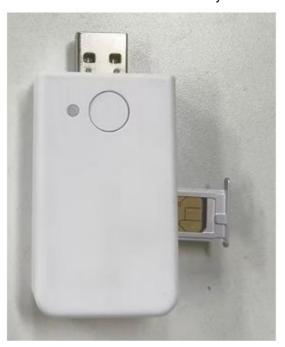
2. The SIM card is inserted into the slot with the chip up as shown.
