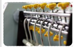
Bend-resistant cable, withstanding more than 400,000 tests
