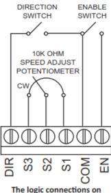
The logic connections on TB501 are isolated up to approximately 4 kV.
