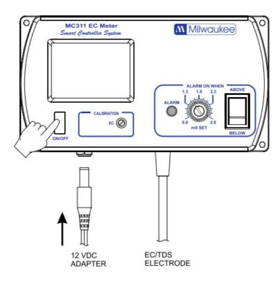
**NOTE:** The output power contact has no protection fuse inside the meter. It is recommended to protected it outside, against failure.
