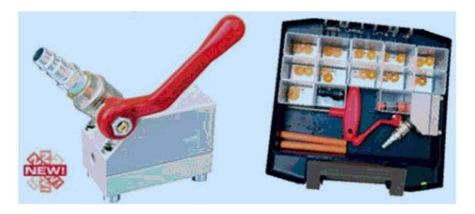
The mini blowing junction block is used for straightening a cable when blowing in two directions, and when there is a loop left because the regular blowing machine does not fit into the excavation (see illustration below). It is the perfect accessory for a MiniFlow RAPID.
