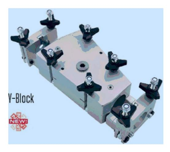
The V-block, used for overblow, can assist you in adding one cable to an existing duct where another cable is installed. Its surface is treated aluminium and it can withstand airtwater pressure up to 25 bar.
