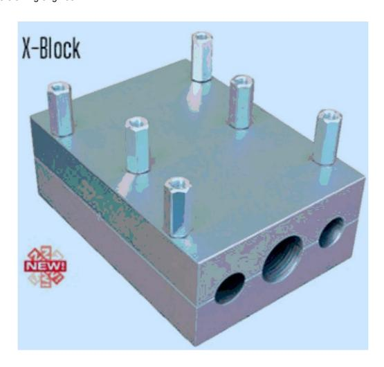
The X-block is used for adding one cable to an existing duct with two cables inside. It is made from surface treated aluminium and can easily withstand a pressure of 25 bar from air/water-
