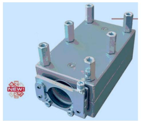
The duct joining block is used for joining ducts in almost all combinations between 14 and 50 mm. Unlike a plastic connector, the joining block can be split into two halves and used again and again. At the same time it can withstand much greater pressure. It's made from surface treated aluminium and can easily withstand a pressure of 25 bar from air/water.
