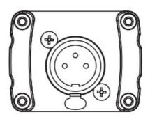
INPUT: XLR input socket OUTPUT: XLR output socket
