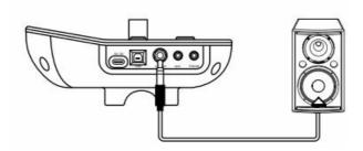
Connect the inputs of your mono amplifier, active monitor, mixing console or recording device to the [L/MONO] output sockets of the drum module.
