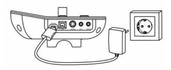
Connect the included power adapter to the [DC 5 V] input on the rear panel of the drum module and then put the power plug into the power outlet.
