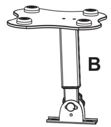
C) Fix the base plate with  $2 \times \text{hexagon bolts}$  at the lower end of the support arm. Tighten the screws with the Allen key.
