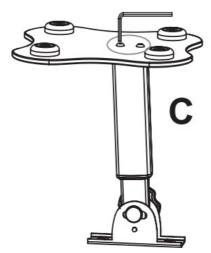
D) Position the speaker plate over the upper end of the support arm. Fix it with  $2 \times \text{hexagon bolts}$  at the upper end of the support arm. Tighten the screws with the Allen key.
