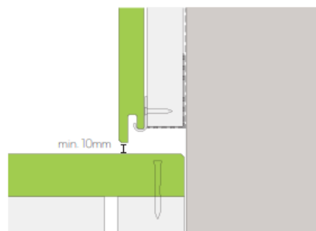
Fig. 5 - Install detail above deck
