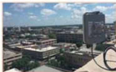
Point-to-Point Broadband Next generation point-to-point broadband links over 2Gb/s, 1 mile, under $200 per node
