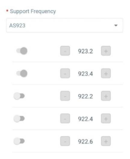
If device frequency is one of CN470/AU915/US915, you can enter the index of the channel that you want to enable in the input box, making them separated by commas.
