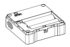
Note: The device can only be powered by ER14505 Li-SOCI2 batteries.
