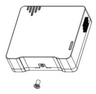
2. Paste 3M double-sided tape to the back of the device, then tear the other side off and place it on a flat surface.
