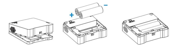
Note: The device can only be powered by ER14505 Li-SOCl<sub>2</sub> batteries.
