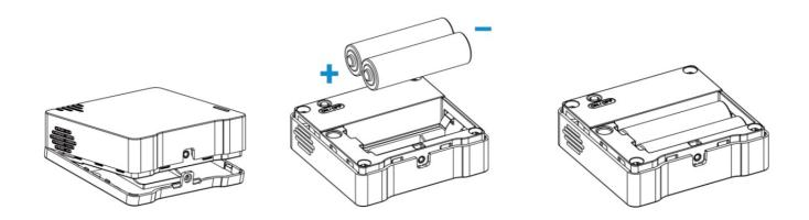
Note: The device can only be powered by ER14505 Li-SOCb batteries.
