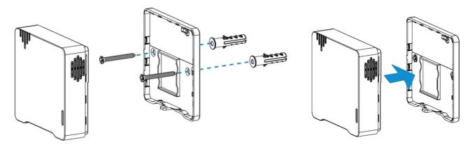
2. Fix the bottom of the device to the rear cover with the theft-deterring screw.
