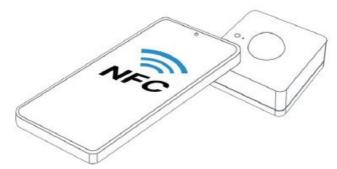
5. Basic information and settings of the device will be shown on ToolBox if it's recognized successfully. You can read and configure the device by tapping the Read/Write device on the App. In order to protect the security of the device, password validation is required when configuring via a new smartphone. The default password is 123456.
