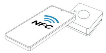
5. Basic information and settings of the device will be shown on ToolBox if it's recognized successfully. You can read and configure the device by tapping the Read/Write device on the App. In order to protect the security of the device, password validation is required when configuring a new smartphone. The default password is **123456.**
