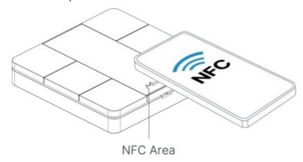
5. Basic information and settings of the device will be shown on Tool Box if it's recognized successfully. You can read and configure the device by tapping the Read/Write button on the App. In order to protect the security of devices, password validation is required when first configuration. The default password is 123456.
