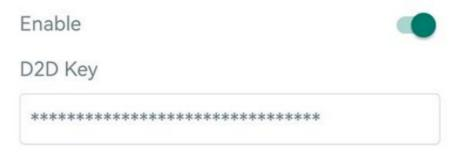
2. Enable one of WS136 & WS156 button mode and configure a 2-byte hexadecimal command (This command is pre-defined in Milesight D2D agent device). When you press this button, WS136 & WS156 will send the control command to corresponding Milesight D2D agent devices.
