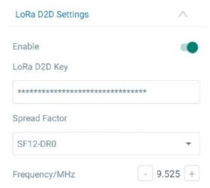
3. Enable one of the WS101 button modes and configure a 2-byte hexadecimal command (This command is predefined in LoRa D2D agent device). When you press as this button mode, WS101 will send the control command to corresponding LoRa D2D agent devices.
