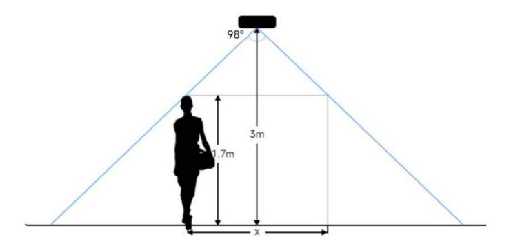
For example, if the Minimum height of pedestrians is 1.7 m, the detection area corresponding to each installation height is as follows:
