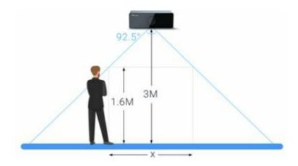
The detection area covered by the 3D ToF People Counting Sensor is related to the field of view angle of the device, the installation height and the target height. The length of the detection area is approximately x=2. I x(H-hmin) and the width of the detection area is approximately  $y=1.32 \times (H-hmin)$ .
