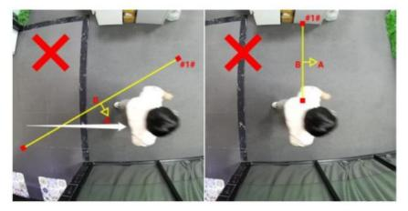
3. A redundant identification area needed to be left on both sides of the detection line for the target. This is to ensure that the sensor has stable recognition and tracking of this target before it passes the detection line, which will make the detection and count more accurate.
