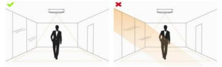
Make sure there are no moving objects interfering in the counting area. For example, do not install the sensor too close to a door.
