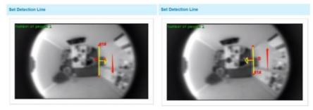
2. Ensure that the detected target can pass through the detection line completely. It's recommended that the detection line is perpendicular to the In/Out direction and on the center of detection area without other objects around.
