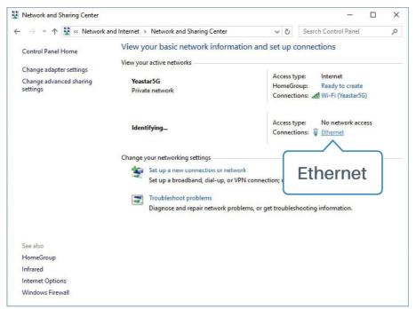
Go to "Properties" → "Internet Protocol Version 4 (TCP/IPv4)" and select "Use the following IP address", then
