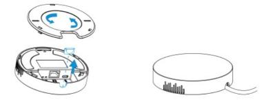
• Align the mounting plate horizontally to the desired position on the wall or ceiling to mark two mounting holes, drill two holes as these marks, insert wall plugs into the holes respectively.
