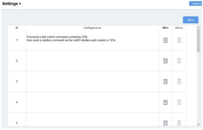
2. Set an IF condition based on the terminal device data or UC100 device status.
